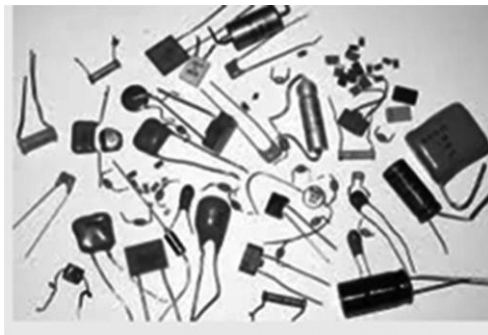
Fig. 21. Capacitors as devices for electric circuits.
