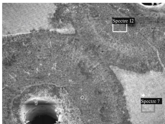
Figure 1. SEM image of the collector's surface (secondary electron detection mode) at 20 keV beam energy [10]
