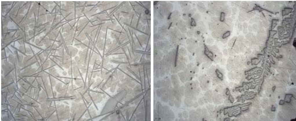
Figure 1. The distribution of intermetallics particles in the master alloy.
