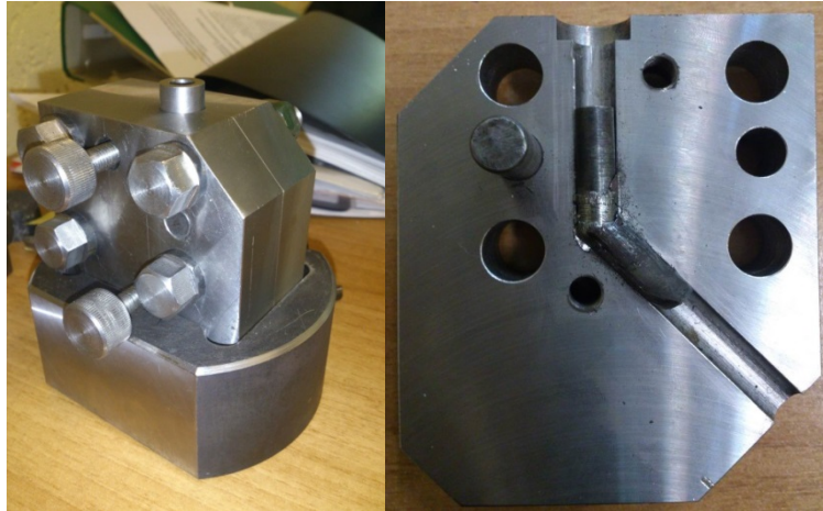
Figure 1. Devices for giving bulk samples of metals sub-nano-crystalline structure (a) and the inner surface of the sample matrix with the punching steel (b) is illustrated.
