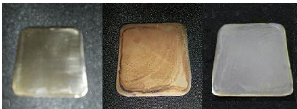
Figure 1. Left: panel with deposited gel prior to drying, Middle: panel with ZnO film after drying at 250^\circ\text{C} ; Right: panel with ZnO film after sintering at 550^\circ\text{C} .
